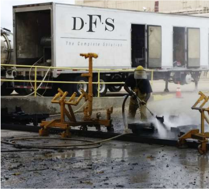
ABOVE: Blasting of chassis carts with 40k PSI hydro-blaster.
